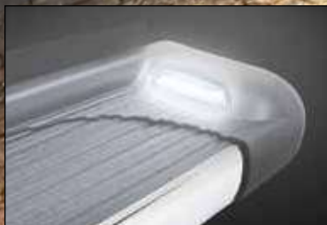
WATER-RESISTANT LED LIGHTS ILLUMINATES STEP SURFACE
